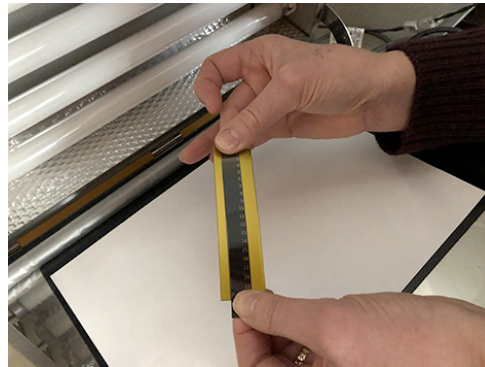
21-step Stouffer Wedge on Miraclon DS94 photopolymer plate, about to be placed in a UV exposure unit with florescent lamps, and vacuum with diffusion film.
